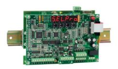
It is a regulator of tension which uses the partialisation principle (cut phase) which is totally controlled on 3 phases for the partialisation of rms tension on asynchronous triphase motors mounted on heat exchangers.
