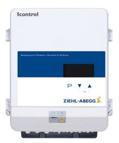
The device is a tension speed controller which uses the partialisation principle (phase cut), totally controlled on 3 phases. It is used for the partialisation of the rms tension in asynchronous triphase motors mounted on heat exchangers.
