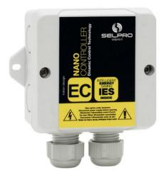
The EC NANO speed controller is a digital multifunction unit with a microprocessor, which can simultaneously and coordinately control different EC fans, using signals coming from the programmable analog inputs, which are suitable to read the signals produced by temperature (°C), pressure (bar) and flow rate (mc) transducers.
