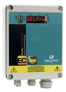
The EC PLUS speed controller is a digital multifunction unit with a microprocessor, which can simultaneously and coordinately control different morotized actuators, using signals coming from the three programmable analog inputs, which are suitable to read the signals produced by temperature(° C), pressure (bar) and flow rate (mc) transducers.
