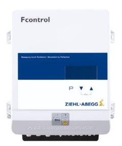
The device is a regulator of tension which uses an inverter for the partialisation of rms tension on asynchronous triphase motors mounted on heat exchangers for climatization and refrigeration plants.
